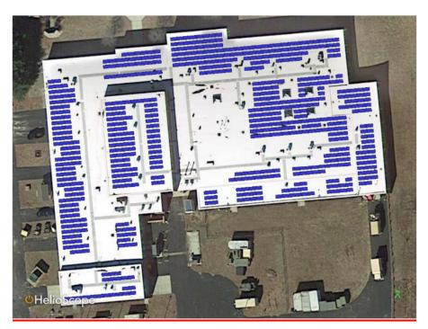
DC Capacity (kW) – 207.5 AC Capacity (kW) – 216.5 No. Modules – 647 Module - Trina Solar 320 Watt Inverter - SMA 24000TL-US Est. Annual Solar Production (kWh) – 281,200 Avg. Annual Energy Consumption (kWh) – 316,300 Full details on the study can be found in Exhibit "A": Camp Fogarty Regional Training Site Solar PV Technical and Economic Feasibility Memorandum.
