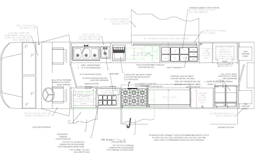
DUE TO THE TWO SEPA RATE POWER SO URCES (GENERA TORS). TWO SEPARATE ELECTRICAL PANELS WILL BE INS TALL ED THAT WILL OPERATE INDEPENDENTLY FROM ONE ANO THER
